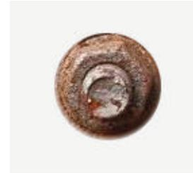
Many companies use only galvanized or zinc coated fasteners that can rust and void the steel mill roof warranty. Others use an alloy cast head that may prevent red rust, but are prone to oxidize and discolor to black or grey which streaks the roof panels. This unsightly appearance will require the roof to be painted.
