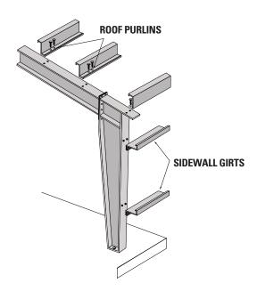
Ironbuilt secondary framing, girts and purlins as a standard have hot dipped galvanized coating. This prevents the components from bleeding or dripping rust. Standard red and grey primer or custom coatings are also available if required.
