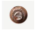
Many companies use only galvanized or zinc coated fasteners that can rust and void the steel mill roof warranty. Others use an alloy cast head that may prevent red rust, but are prone to oxidize and discolor to black or grey which streaks the roof panels. This unsightly appearance will require the roof to be painted.
