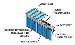
The connection point of the wall and roof sheeting at the eave is specially designed to create a super tight seal. An outside foam closure applied at the top of the wall fits the corrugation of the wall sheeting and an inside foam closure sits on top of the eave strut sealing the roof sheeting for a weathertight seal and protection against leaks.
