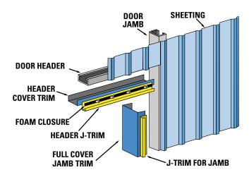
Ironbuilt's door openings come factory ready with the most complete trim and closure system offered anywhere. "J" trim is supplied for the cut edges of the wall sheeting around the door opening. Header cover trim and jamb cover trim enclose the door framing members so no exposed red iron framing can be seen. The door opening trims match the building trim and make the building look fantastic.
