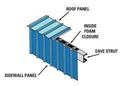
Some companies only use one inside closure and do not use a wall foam closure, and, in some cases do not use a metal eave trim to save money. This allows for penetration by insects, rodents and leaks that can rot the insulation.
