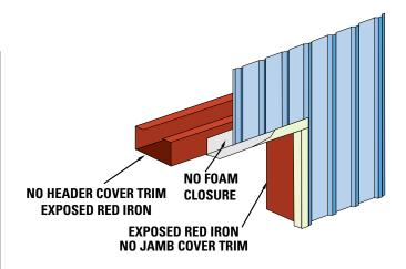
Most other companies do not supply jamb or header cover trim and only supply the "J" trim for the cut edges of the sheeting at the opening. Since the jambs and header are exposed and only have a red-oxide primer, they eventually rust and it runs onto the wall sheeting and concrete floor which looks unsightly.
