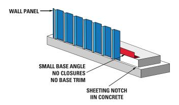
Many companies do not include a base trim which requires the customer to use an expensive notch in the concrete around the perimeter. The base angle is often only 2"x2" and not full sized, does not offer dent protection and is not galvanized which promotes rusting. Other companies use a flimsy lightweight, 20 gauge one-piece base trim that is inferior as it is not as strong and does not seal as well against driving rain.
