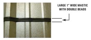
Ironbuilt uses an oversized 1" wide, butyl rubber mastic tape as sealant between every roof panel. The tape has two large beads on it to form an additional water tight seal. When screwing the panels together, the oversized 1" width ensures the roof fasteners will not miss the mastic. The fasteners easily screw down through the mastic for a super tight seal.
