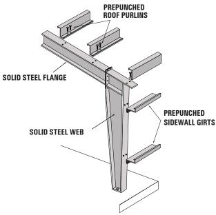
Ironbuilt Structural I-beam frames are made from only 100% USA steel. The flanges are fabricated from solid steel bar stock and the web of the column beams and the rafter sections are made from solid steel plate. For added rigidity, the flanges are made with a minimum of ½" structural plate.
